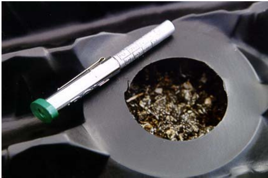
Figure 7 Stress concentrations on the media panel
