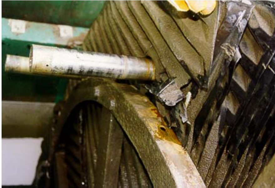
Figure 4 Loss of clamping efficiency resulting from a fractured 'U' strap
